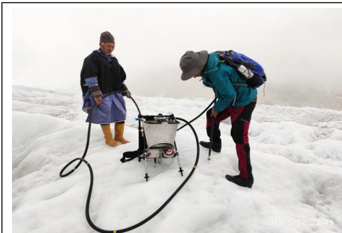
Fig :Drilling of glacial ice using stem drilling machine
