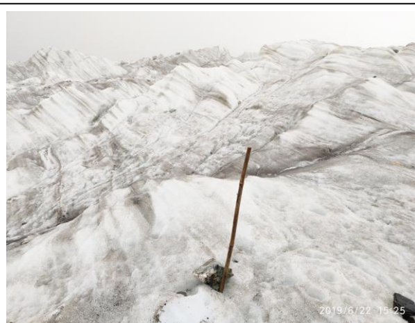
Fig : Stake fixation in lower ablation zone of East Rathong Glacier
